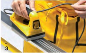
ill. 3) Strip the wax. After about an hour, use the Plexi blade to strip the base in the direction of travel.
